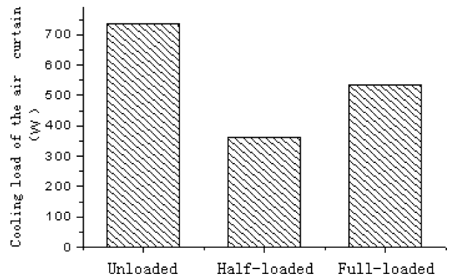
Fig. 16. Cooling load of the air curtain with different filling levels.
